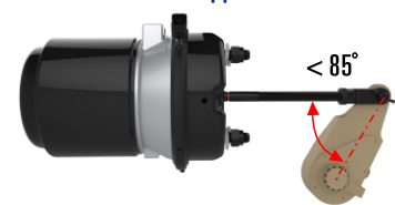
INCORRECT INSTALLED
